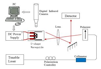
Fig. 2. Schematic of the experimental setup for measuring the transmission spectrum of the resonators and to measure the optical scattering for the feedback control process.
