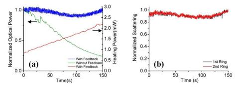
Fig. 6. The active feedback control process. (a) Normalized optical transmission with (the blue line) and without (the green line) the feedback control process. The red line shows the power applied on the heater. (b) The normalized scattering signal for the two rings during the control process.
